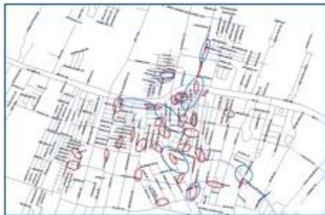
Nearest neighbor hierarchical ellipses map illustrating patterns of crashes in red and patterns of property crimes in blue. Hotspots are identified where the two overlap.
